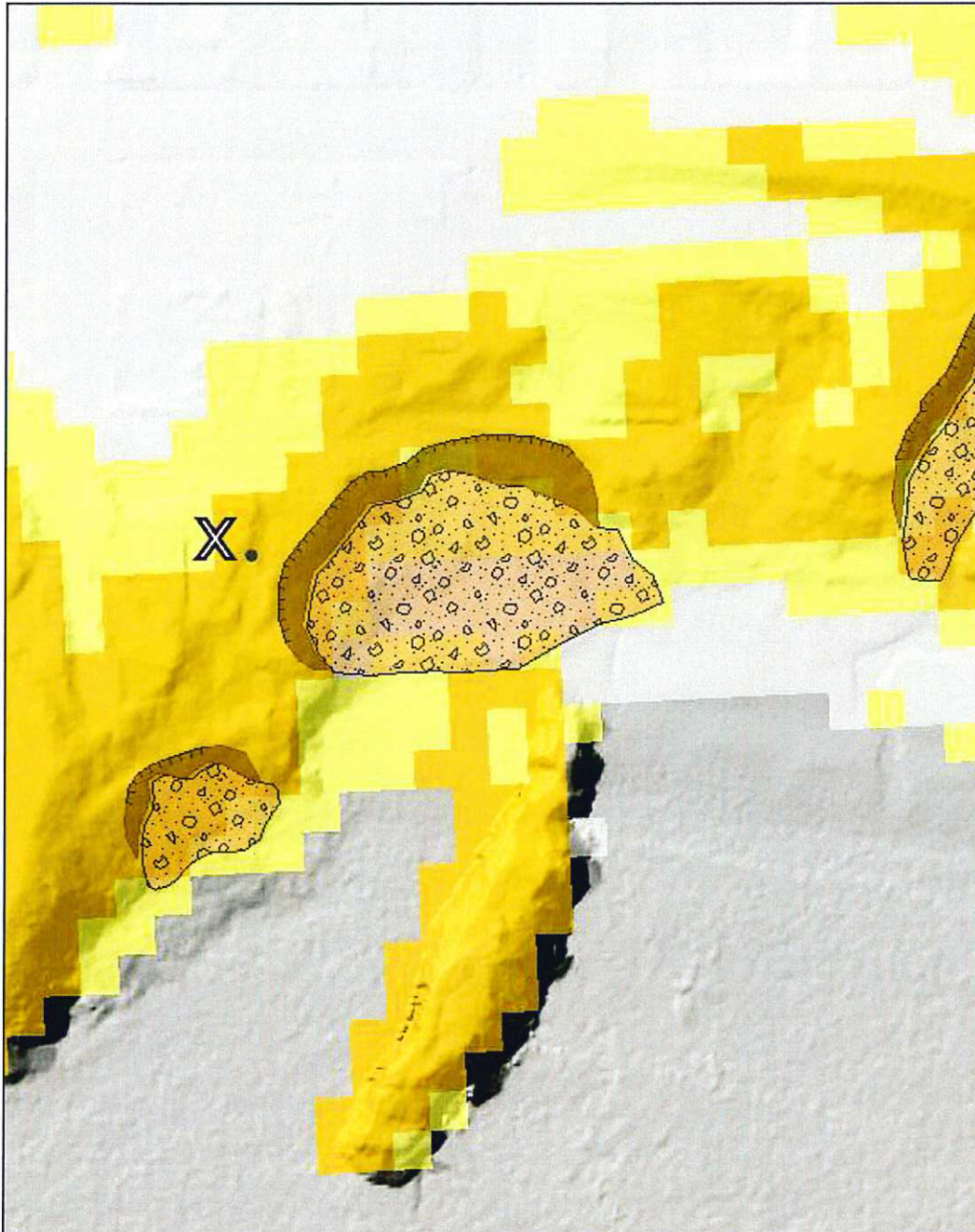
Figure 5. SLIDO map of landslide susceptibility (the risk of landsliding mapped at a regional scale). Gray is Negligible risk; yellow is Low risk; and orange is Moderate risk. The risk assessment is too high under static conditions. The X is the approximate building area.
